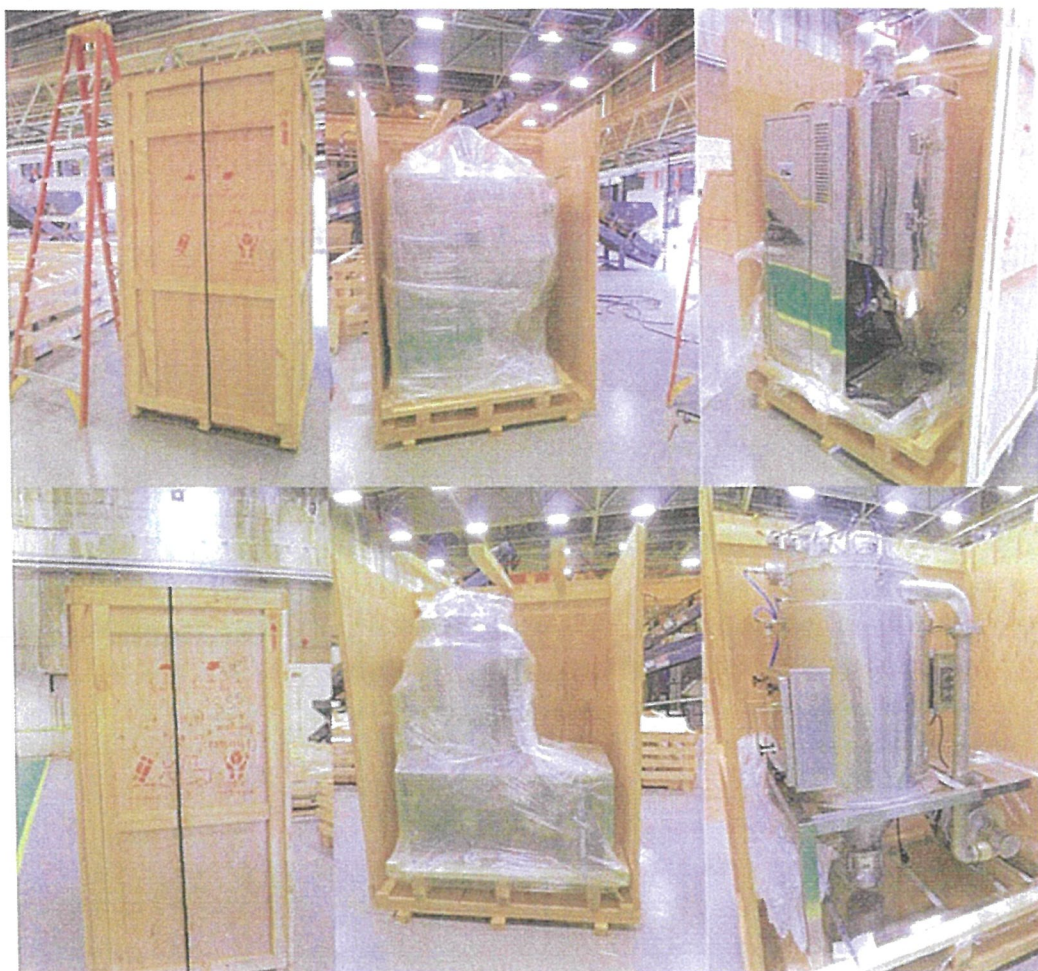
Figure 6.D. Spray dryer removed from shipping crate and shrink wrap following delivery. Top three images: the drying chamber, heater, and control unit. Bottom three images: the fine particulate system. This shipment also featured a third crate containing 8-10 cardboard boxes of parts.
