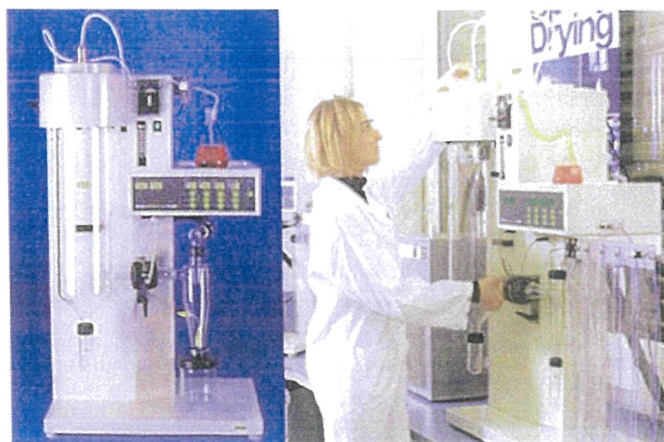
Figure 6.B. Controlled spray dryers. These spray dryers have water evaporation capacities of ~1 kg/hr.
